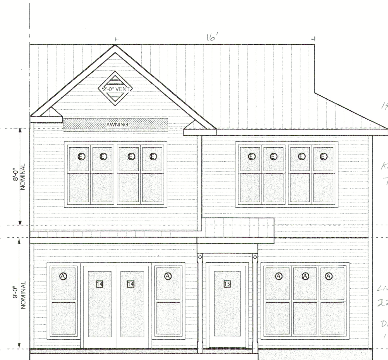
1460 S.F. UNIT PLAN - SOUTH ELEVATION EAST END UNIT - FRONT ENTRY ON SOUTH SIDE scale: 1/4" = 1'0"
