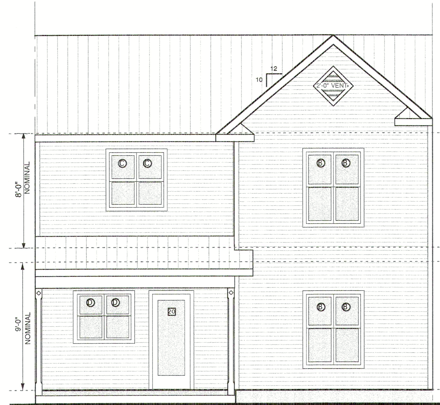
1460 S.F. UNIT PLAN - NORTH ELEVATION MIDDLE UNIT - FRONT ENTRY ON SOUTH SIDE scale: 1/4" = 1'0"
