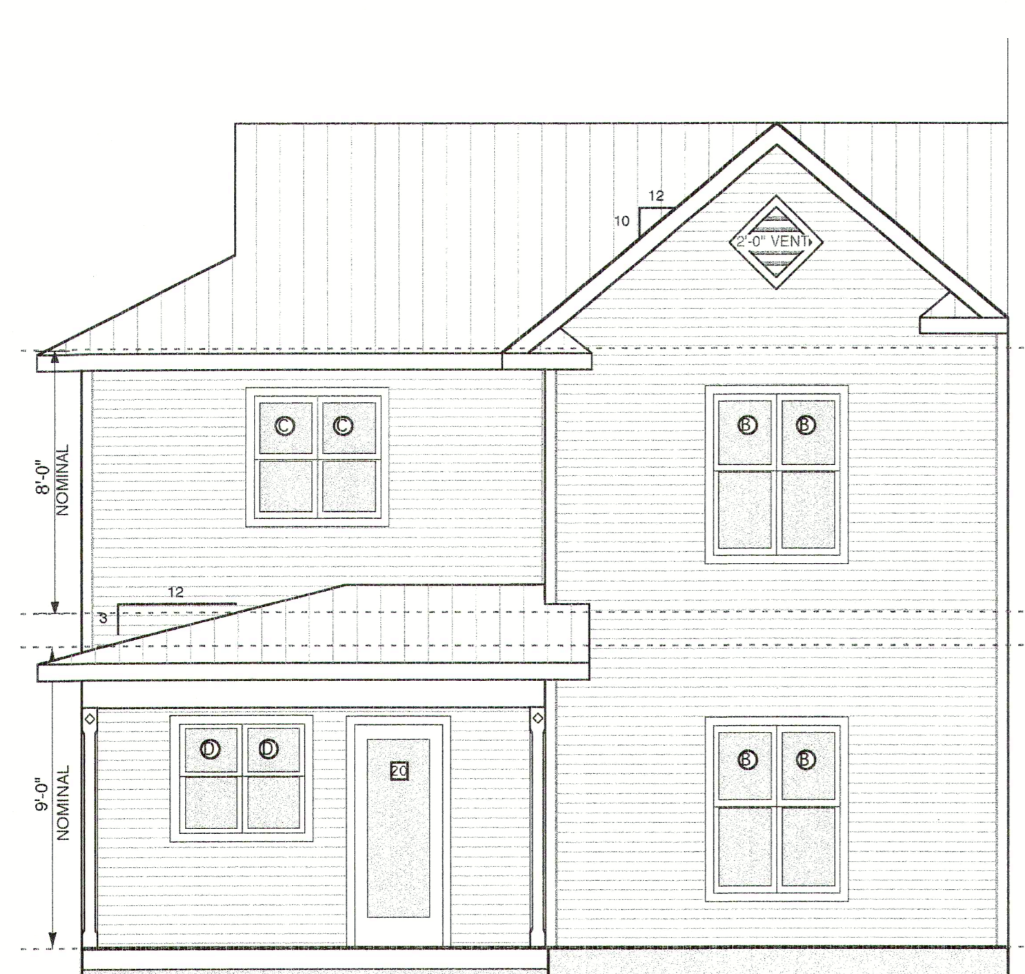
1460 S.F. UNIT PLAN - NORTH ELEVATION EAST END UNIT - FRONT ENTRY ON SOUTH SIDE scale: 1/4" = 1'0"
